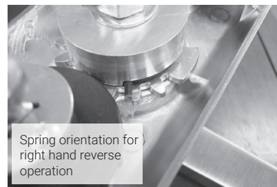
Right Hand Reverse gear & spring orientation
