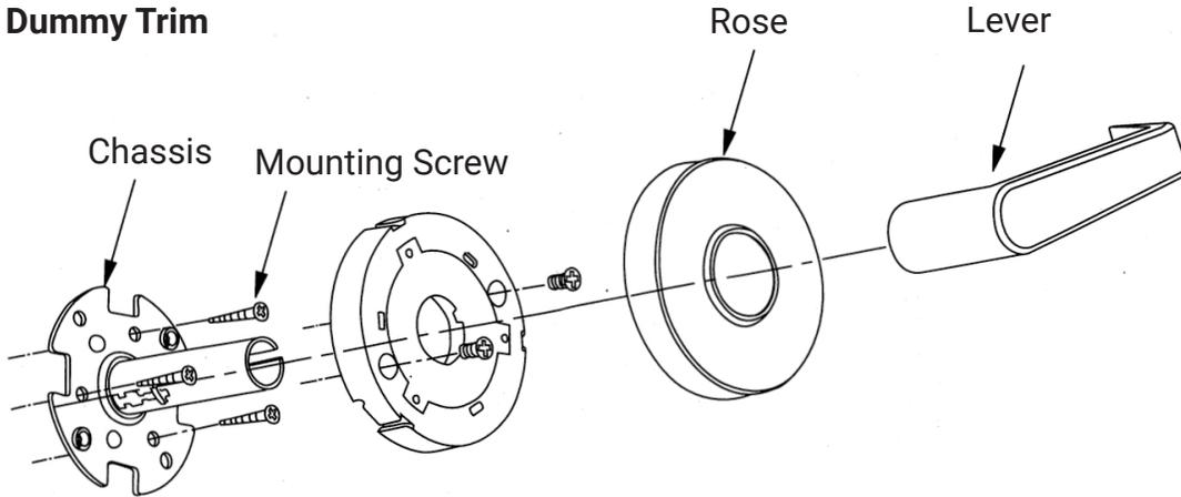
1. Install chassis at proper position on the door by provided three mounting screws.
