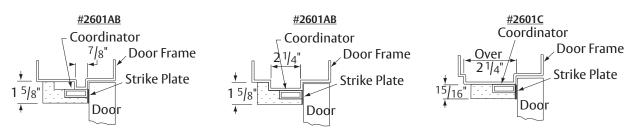
NOTE: Field adjustment of door closers is required after installation of coordinator to insure against doors closing too fast and changing coordinator mechanism. Field adjustment of coordinator override could be needed.
