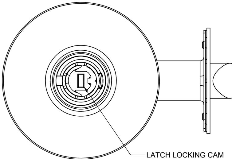
1. USING A SCREWDRIVER, ROTATE THE CAM CLOCKWISE UNTIL THE CAM PROFILE LOOKS LIKE THE PICTURE ON THE LEFT.
