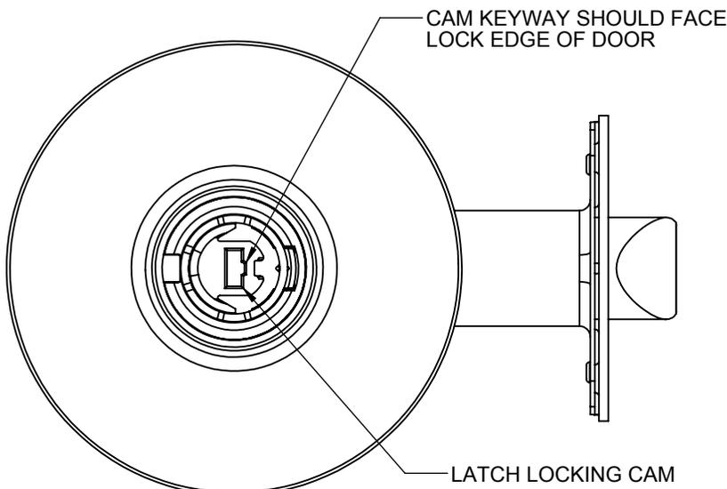
1. USING A SCREWDRIVER, ROTATE THE CAM UNTIL THE KEYWAY FACES THE LOCK EDGE OF THE DOOR.
