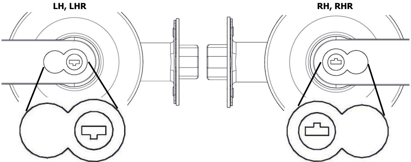
1. USING A SCREWDRIVER, ROTATE THE CAM CLOCKWISE UNTIL THE CAM PROFILE LOOKS LIKE THE PICTURE ABOVE (BASED ON HANDING).
