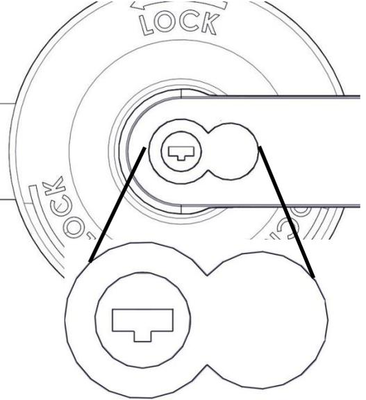
1. USING A SCREWDRIVER, ROTATE THE CAM CLOCKWISE UNTIL THE CAM PROFILE LOOKS LIKE THE PICTURE (BASED ON HANDING AND INSIDE / OUTSIDE).
