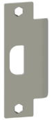
3935 ASA Strike Plate - Standard • 1-1/4" x 4-7/8" (32 mm x 124 mm) • 1-5/16" lip • Other lengths available upon request
