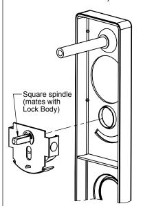
Square Spindle should be in the center of the escutcheon hole.
