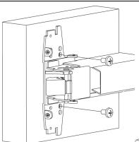
device chassis. Mount exit device using the two the template.
