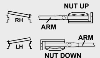
1. Install hold-open foot/nut. Left Hand (LH) door = Nut points down. Right Hand (RH) door = Nut points up.
