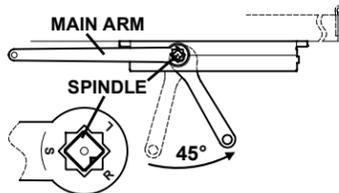
4. Rotate closer spindle 45° towards hinge / pivot.
