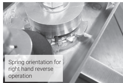
Right Hand Reverse gear & spring orientation
