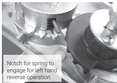
Spring orientation for right hand reverse operation
